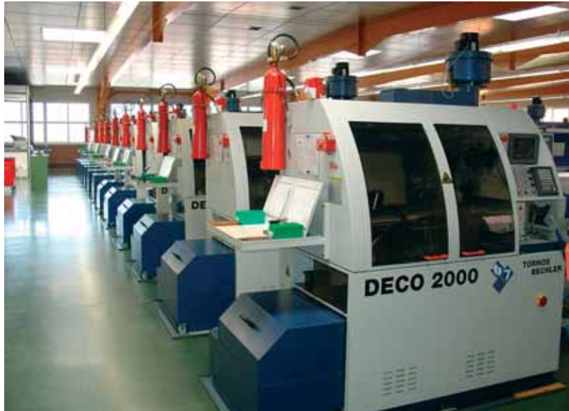
At MGB, all machines are equipped with facilities aimed at making the production environment safe, e.g. fire extinguishers.
